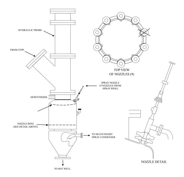
Secondary spray condenser (containing NEW equipment)
